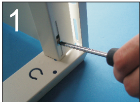
Remove the door from the frame
